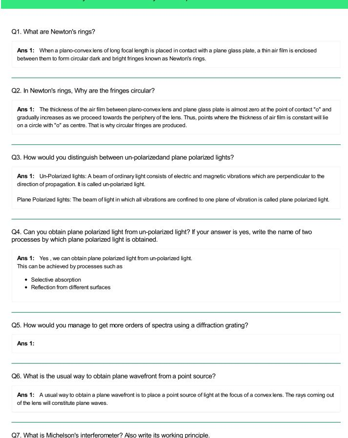
Ans 1: Michelson's interferometer is an instrument that is capable of measuring distance with extremely high precision.
