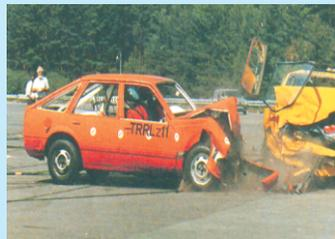
During an accident, crumple zones collapse. This increases the impact time by providing extra time for crumpling. The impact of force is highly reduced and saves the passengers from severe injuries.
