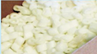
Air enclosed in the cavities of these materials makes them flexible and soft. During any mishap, they increase the impact time on fragile objects. An increase in impact time lowers the rate of change of momentum and hence lessens the impact of force. This lowers the possible damage due to an accident.
