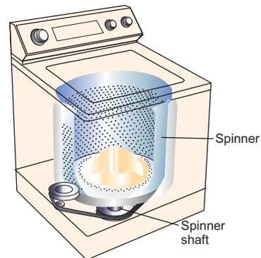
**Figure 3.30:** Dryer of washing machines has perforated wall.
