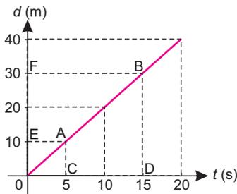
**Figure 2.19:** Distance time graph showing constant speed.
