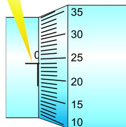
**Figure 1.12:** Zero error of the screw gauge
