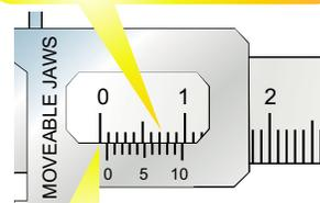
Zero error is positive as zero line of vernier scale is on the right side of the zero of the main scale.
