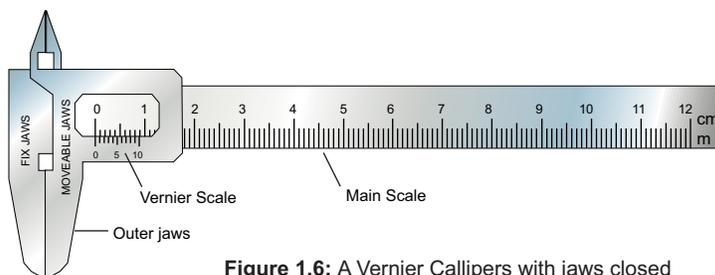
Figure 1.6: A Vernier Callipers with jaws closed
