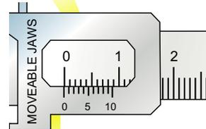
Zero error is negative as zero line of the vernier scale is on the left side of the main scale.
