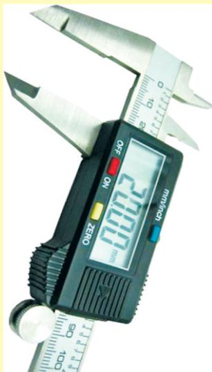
Digital Vernier Callipers has greater precision than mechanical Vernier Callipers. Least count of Digital Vernier Callipers is 0.01 mm.
