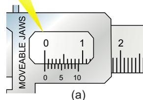
Zero error is  $(0+0.07)$  cm as 7th line of vernier scale is coinciding with one of the main scale division.
