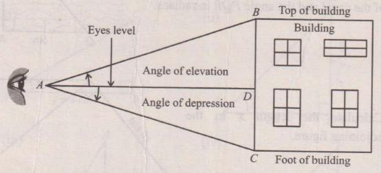
The angle between the horizontal line AD (eye level) and the line from the eye 'A' to the foot of the building (C) is called the angle of depression.
