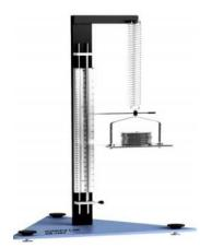
Fig 5.4 Extension in the spring depends upon the load.
