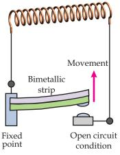
Fig 9.10 Bimetalic Thermostat
