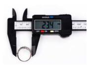
Fig 1.15 Digital vernier calipers
