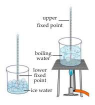
Fig 9.4 Heating ice experiment
