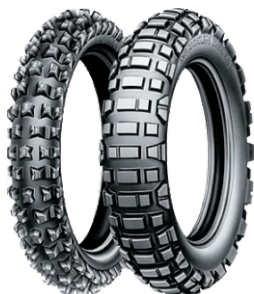
Figure 3.20: Threading on tyres provides good road grip.
