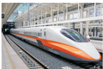
Figure 3.23: Streamlining the bullet train reduces air resistance at high speed.
