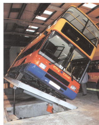
Figure 4.35: A double decker bus being under test for stability.
