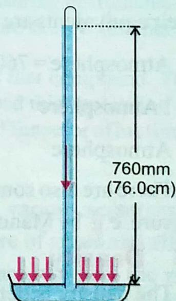
$P_{\text{atm}}$  = Height of "Hg" column in glass tube
