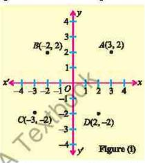
In an Argand diagram, the complex number x+iy is uniquely represented by the order pair (x, y). In Figure (i), the complex numbers 3 + 2i, -2 + 2i, -3 - 2i and 2 - 2icorrespond to the order pairs (3, 2), (-2, 2), (-3, -2) and (2, -2) respectively have been represented geometrically by the point A, B, C and D.
