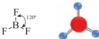
Figure 3.18 \text{BF}_3 is an AB 3 system having triangular planar geometry
